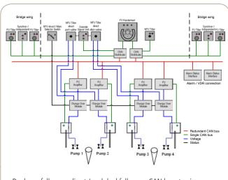
Dual non-follow-up direct / and dual follow-up CAN bus steering gear control system for a vessel with dual rudders
