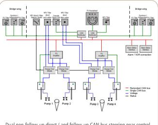
Dual non-follow-up direct / and follow-up CAN bus steering gear control system for a vessel with dual rudders
